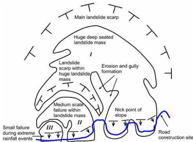
**Fig. 12** Schematic model of valley creeping type landslide terrain in mountains of central Nepal. The road is found to be constructed on toe of large-scale landslides having clay mineralization in failure zone as shown in Fig. 10 and 11. Stage III is associated with the monsoon rainfall related landsliding process
